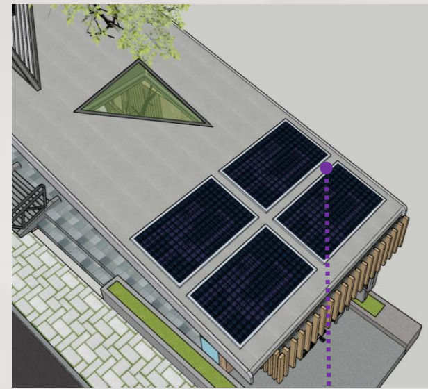
SOLAR CELLS POWER THE VENDING MACHINE, WATER COOLER, DISPLAY PANELS, MOBILE CHARGING
